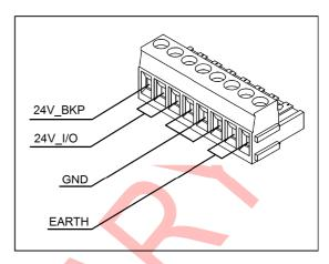
Please notice the presence of a separated earth contact, used to connect the shield of the I/O cables and for EMC filtering purposes.
