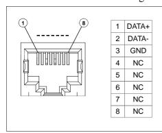
buses should be done using standard CAT 5E Ethernet cable and RJ45 connectors; the pinout of the Modbus RTU connector is depicted aside.
