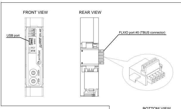
port on the front panel for programming and diagnostic purposes.
