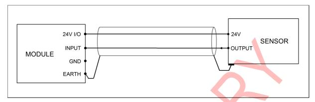
Whenever an input, configured to read currents, absorbs a current out of range, it switches in voltage mode and a warning is issued; this strategy is adopted to avoid damaging of the circuitry and also of the external devices (e.g. when 24V is shorted on an input or when connecting a  $0 \div 10 \text{ V}$  sensor instead of the correct one).
