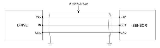
However, if the operating environment is affected by significant electrical noise or the distances to be crossed are significant, the use of a shielded cable may be necessary. In this case, the shield must be connected to earth on both sides, preferably with low-impedance connection, such as a metal cam; the shield is totally ineffective if it is left floating.
