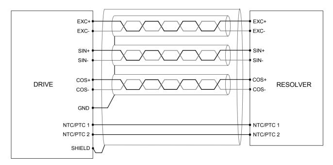
The recommended connection scheme for the resolver is shown in the following picture:
