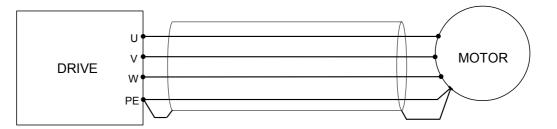
Due to the high noise levels generated by PWM modulation on the motor outputs, it is obligatory to use a shielded cable for connecting motors. The shield must be connected to earth on both sides with a low-impedance connection (such as a metal cam); using an unshielded cable or a shielded cable whose shield is not connected to earth may generate EMC problems and interference with nearby devices.
