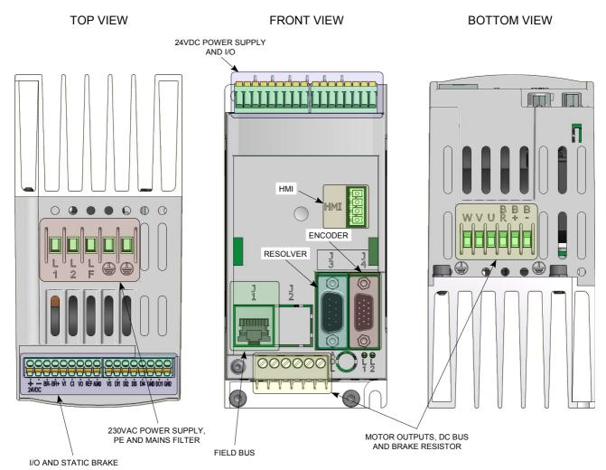
The release code KZ010387 is also equipped with a stage for piloting the brake resistor.
