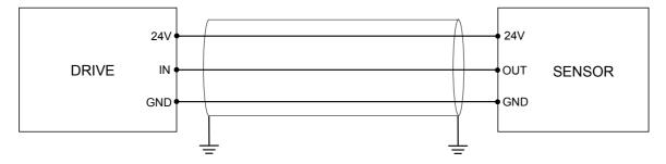
Since the input stage has a relatively wide passband to allow acquisition of high-frequency signals, it is particularly susceptible to electrical interference. Therefore, it is recommended to use a shielded cable for the wiring. In this case, the shield must be connected to earth on both sides, preferably with low-impedance connection, such as a metal cam; the shield is totally ineffective if it is left floating.
