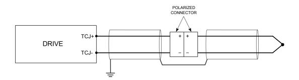
Since the amplitude of the signals delivered by the thermocouple is very low, the signals are particularly susceptible to electrical interference. For this reason, above all when the wiring extends over great distances, it is strictly recommended to use a shielded cable. If an extension cable is used, it is necessary to join the thermocouple shield and the extension cable (see picture).
