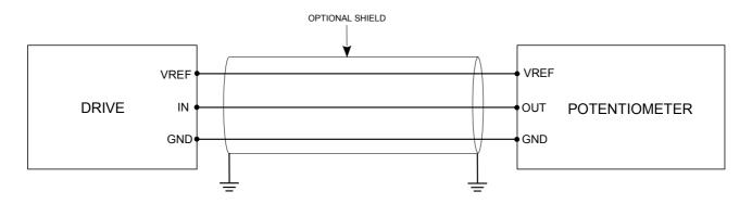
In both cases, it is recommended to use shielded cables for the connections.
