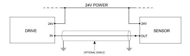
Since 4 to 20mA signals are inherently resistant to electrical interference, the wiring can be made by using unshielded cables in many cases. However, a shielded cable is preferred when the wiring extends over great distances or through particularly unfavourable environments.
