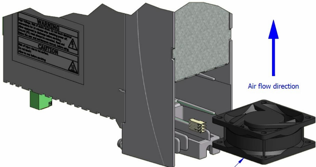
Take the replacement fan (KM021008), connect the connector to the board, then insert it until it engages in the 2 tabs.
